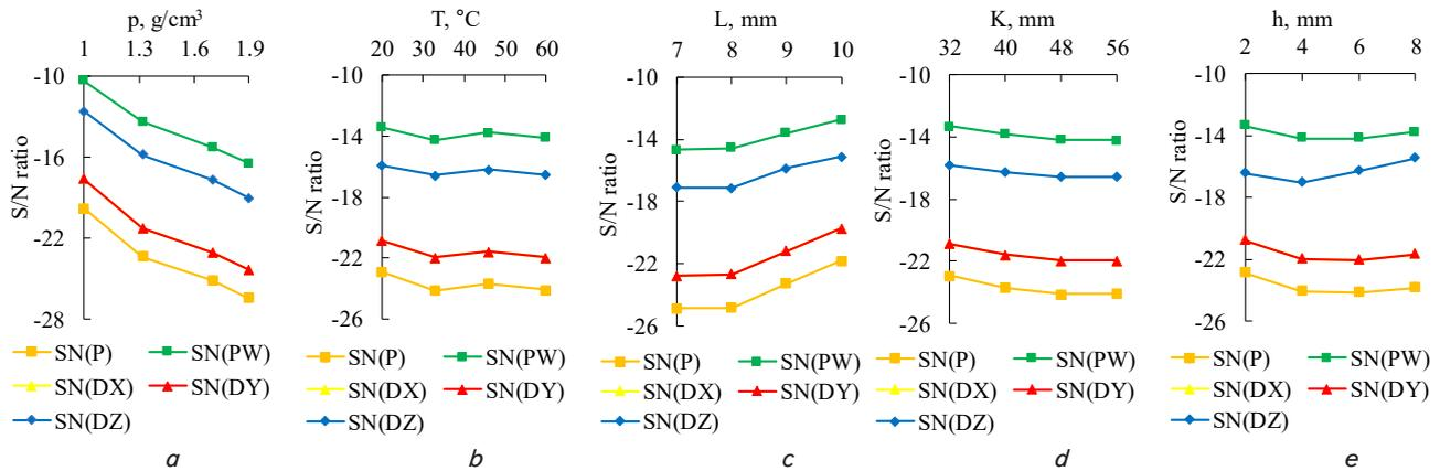
Fig. 7. Influence of the input parameters on the signal-to-noise ratios of the output parameters: *a* – influence of liquid density; *b* – influence of medium temperature; *c* – influence of wall thickness; *d* – influence of the spacing of stiffeners; *e* – influence of stiffeners height
