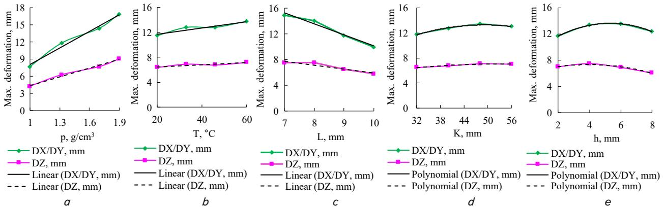
Fig. 9. Influence of the input parameters on the deformations of a PE tank (DX/DY, DZ):
