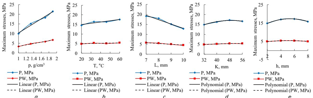
Fig. 8. Influence of the input parameters on the maximum stresses ( $P$  and  $PW$ ): *a* – influence of liquid density; *b* – influence of medium temperature; *c* – influence of wall thickness; *d* – influence of the spacing of stiffeners; *e* – influence of stiffeners height
