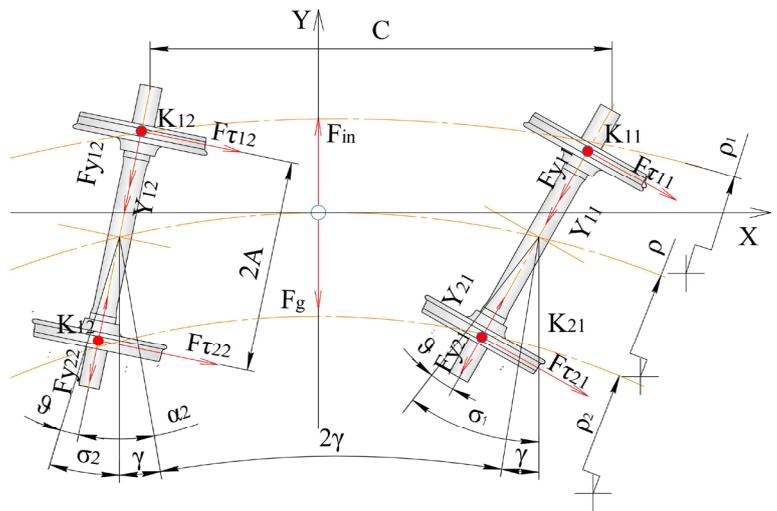
Fig. 3. Scheme of external forces acting on the bogie (projection of forces onto the horizontal plane XOY)
