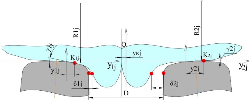
Fig. 2. Contact scheme of the wheelset and rails
