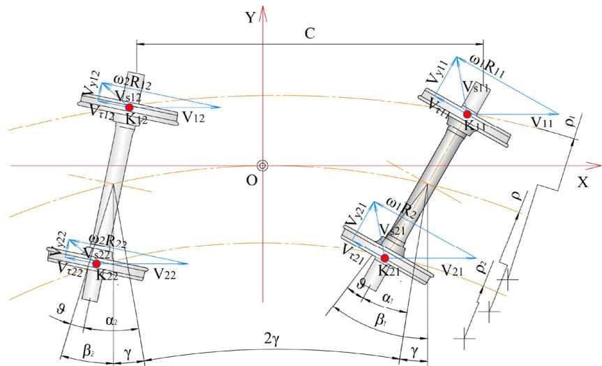
Fig. 1. Kinematic diagram of bogie movement in a circular curve: velocity vectors of the relative movement of the contacting surfaces of the wheels and rails at the points of contact
