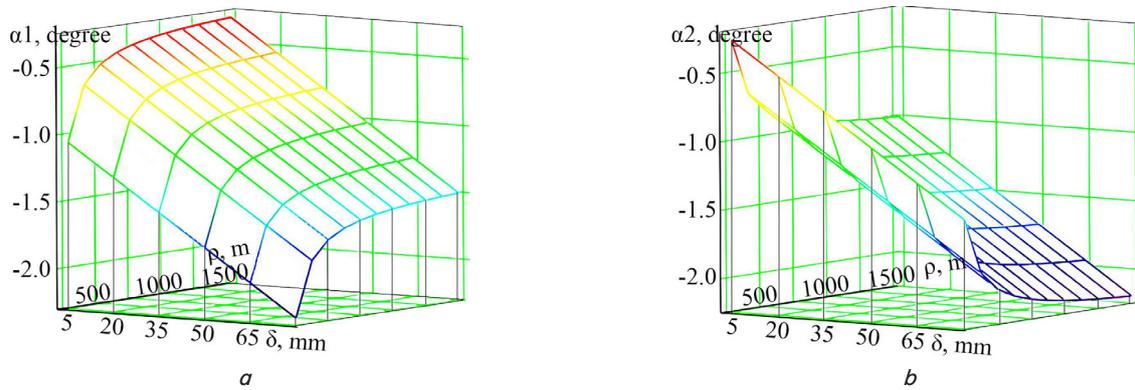
Fig. 6. Dependences of wheelsets approach angles  $\alpha$  (degrees) on track clearances  $\delta$  (mm) and curve radius  $\rho$  (m):  $a$  – 1<sup>st</sup> wheelset;  $b$  – 2<sup>nd</sup> wheelset
