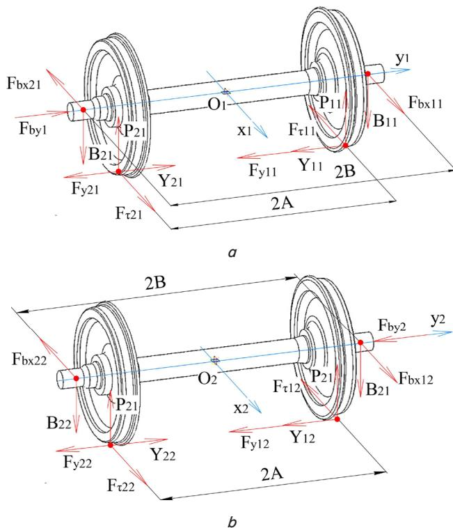
Fig. 5. Scheme of external forces acting on wheelsets from the track and the bogie frame: a – 1<sup>st</sup> wheelset; b – 2<sup>nd</sup> wheelset
