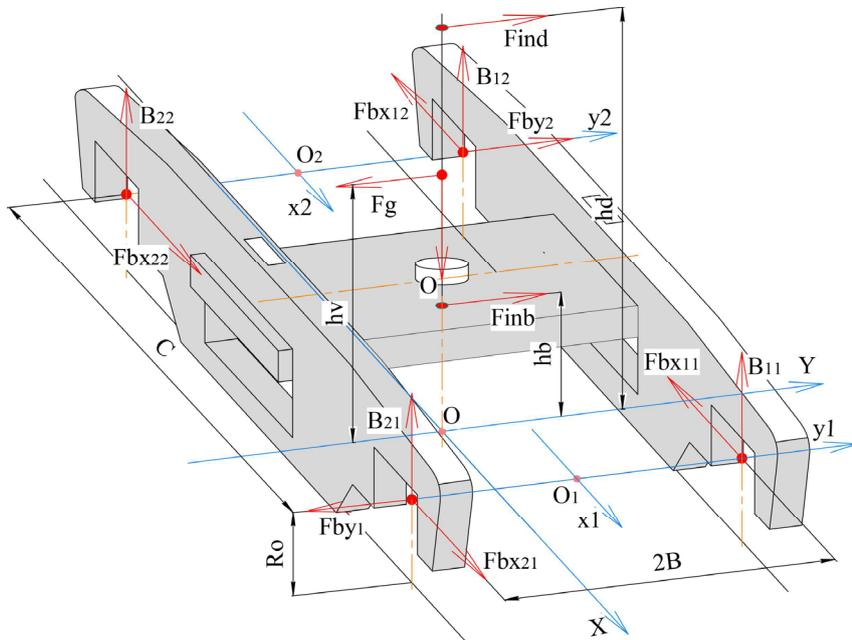
Fig. 4. Diagram of external forces acting on the bogie frame
