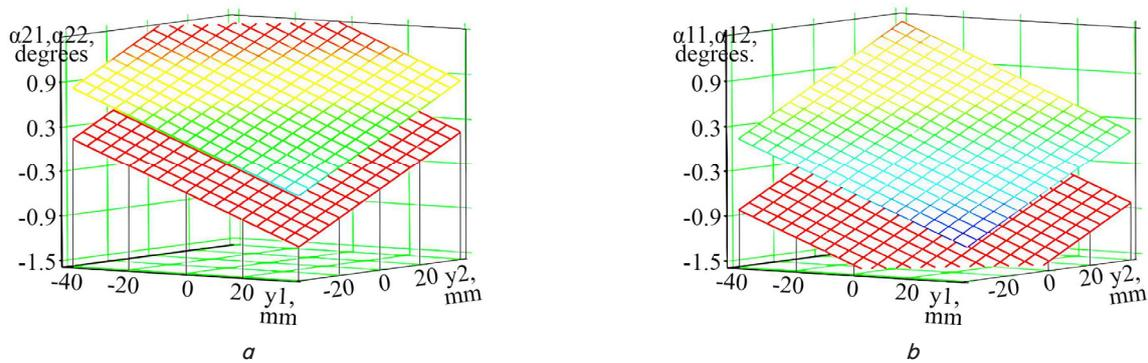
Fig. 7. Dependences of the approach angles of wheelsets  $\alpha_{11} \dots \alpha_{22}$  (degrees) on the transverse movements of wheelsets  $y_1, y_2$  (mm) and the radius of the curve  $\rho$  (m):  $a$  –  $\rho=300$  m;  $b$  –  $\rho=1500$  m
