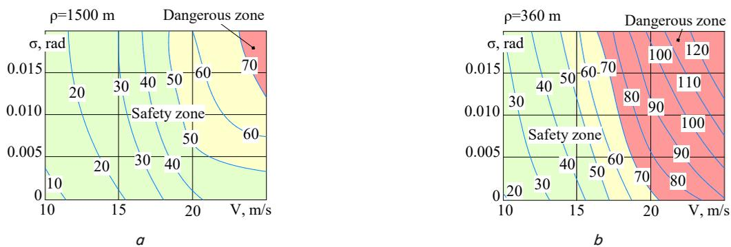
Fig. 8. Dependences of steering forces  $Y$  (kN) on the skew angles of wheelsets in the bogie  $\sigma$  (rad), speed of movement  $V$  (m/s), and curve radius  $\rho$  (m):  $a$  –  $\rho=1500$  m;  $b$  –  $\rho=360$  m
