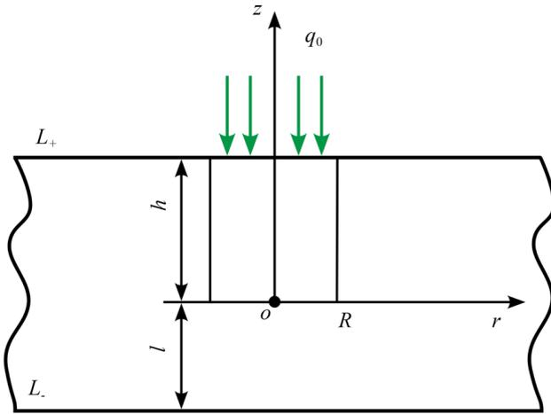
Fig. 1. Section of an isotropic layer with a plane  $\varphi=0$ , which is heated by a heat flow
