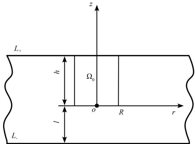
Fig. 2. Section of an isotropic layer with a plane  $\varphi=0$ , which is heated by internal heat sources concentrated in the region  $\Omega_0$
