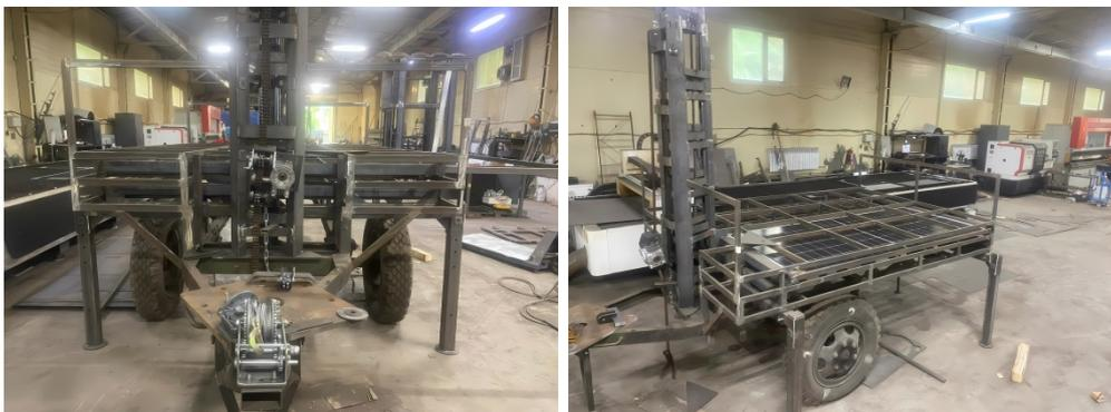
Fig. 9. The assembly process of the full-size mobile wind turbine
