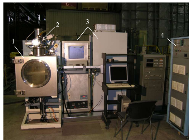
Fig. 1. Experimental setup for electron beam 3D printing: 1 – vacuum chamber; 2 – electron beam gun; 3 – control cabinets; 4 – high-voltage source
