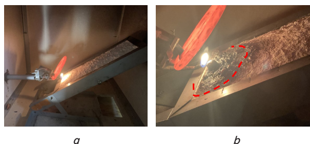
Fig. 7. Results of studies into the process of ignition and flame propagation by insulation with a treated coating: a – the effect of the flame on the sample; b – swelling of the coating (highlighted area)
