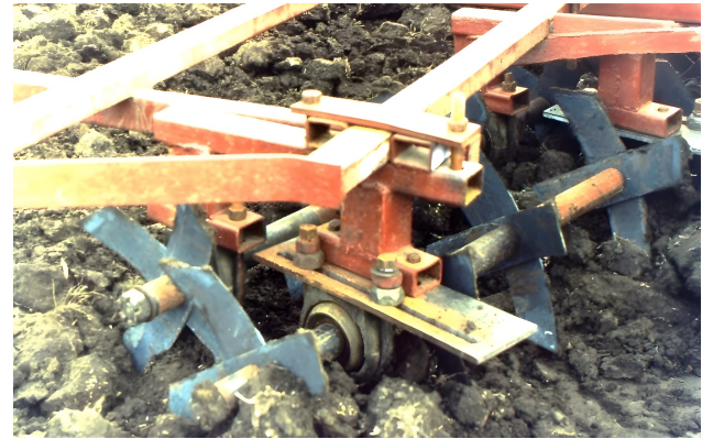
Fig. 3. A general view of the X-shaped rotary working bodies that were used in the experiment
