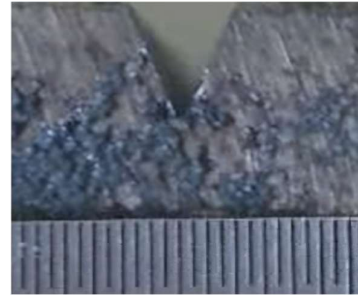
Fig. 3. Groove design triangular prism with a width of 5 mm
