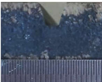
Fig. 2. Groove design trapezoidal prism with a width of 5 mm
