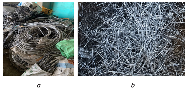
Fig. 1. Raw material for Al electrical cable scrap: a – Al scrap from collectors; b – Al scrap that has been cleaned and cut
