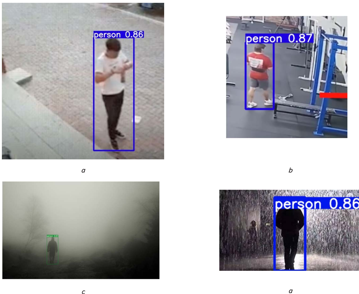
Fig. 10. Human detection: a – outdoor environment; b – indoor environment; c – foggy environment; d – rainy environment
