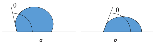
Fig. 4. Contact angle to determine adsorption characteristic between lubricants and surface: a – poor wettability; b – good wettability
