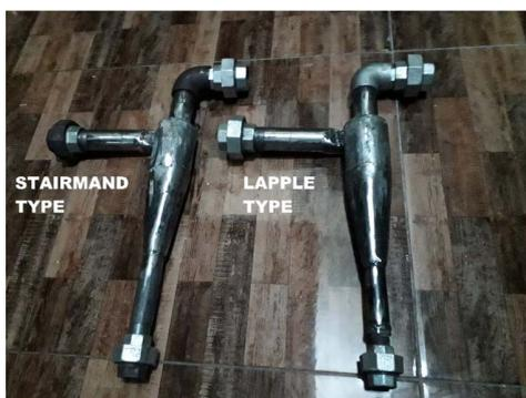
Fig. 2. Two types cyclone separator
