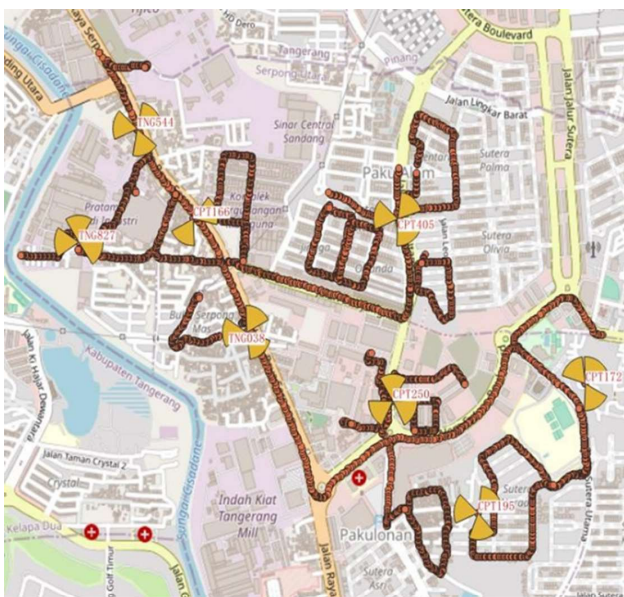
Fig. 4. Fixed wireless access route test by wireless drive test tools
