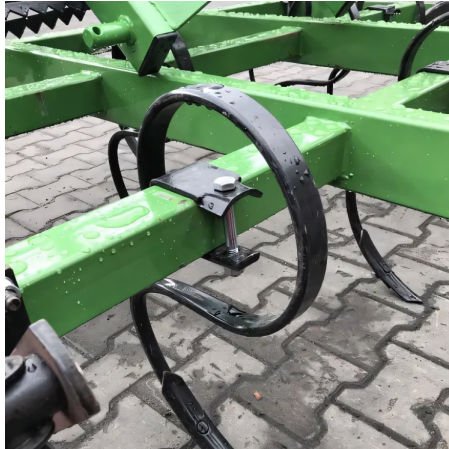
Fig. 2. S-shaped paw riser on the frame of the cultivator
