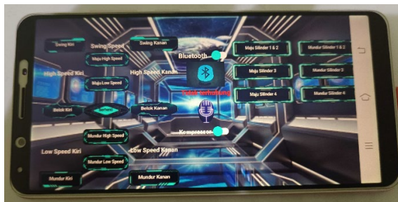
Fig. 4. Wireless remote for new model excavator
