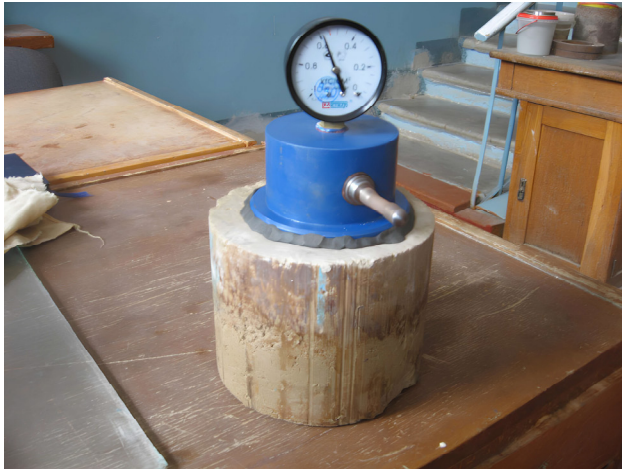
Fig. 3. Methodology for express determination of waterproofness of a soil-cement sample using the VV-2 device
