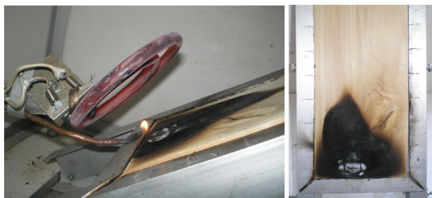
Fig. 7. The process of conducting tests on a wood sample treated with a mixture of aqueous solutions of inorganic salts based on orthophosphoric acid, urea, and oxyethylidenediphosphonic acid
