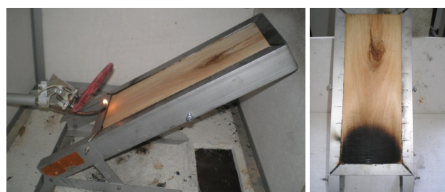
Fig. 6. The process of testing a sample of wood treated with a mixture of an aqueous solution of phosphate and ammonium sulfate
