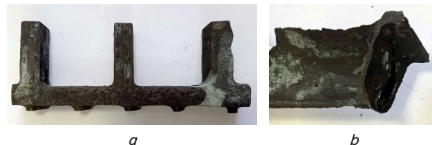
Fig. 1. Turbine elements: a – U-shaped fastener; b – part of the turbine blade
