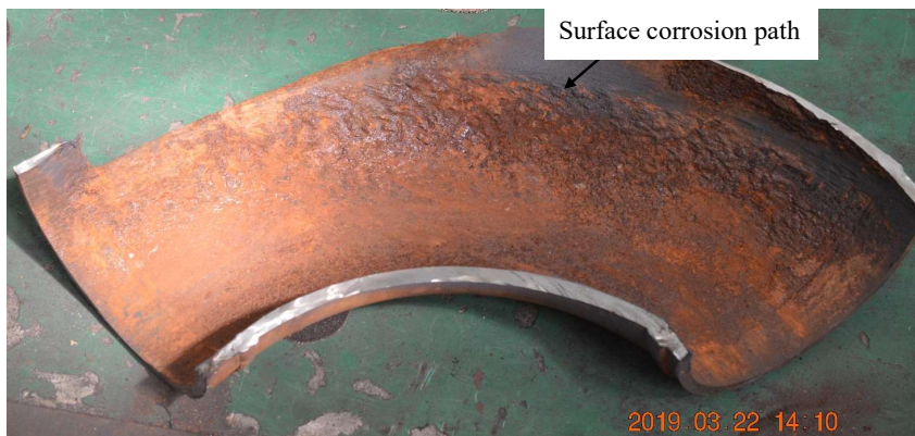
Fig. 4. Surface corrosion path in the defect area
