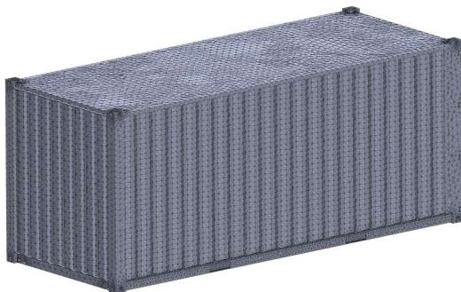
Fig. 7. Finite element model of a container
