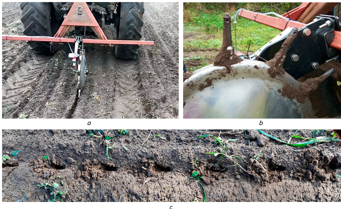
Fig. 4. Investigating the operation of a rotary needle tool under field conditions: a – general view of the installation; b – the effect of soil sticking to the needles; c – appearance of holes in the soil
