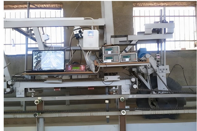
Fig. 2. Installation with a soil bin for measuring parameters in the operation of agricultural wheels [3]
