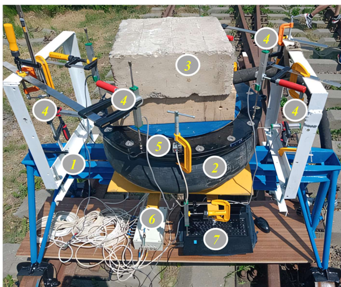
Fig. 3. Dynamic test installation of a pneumatic spring:
