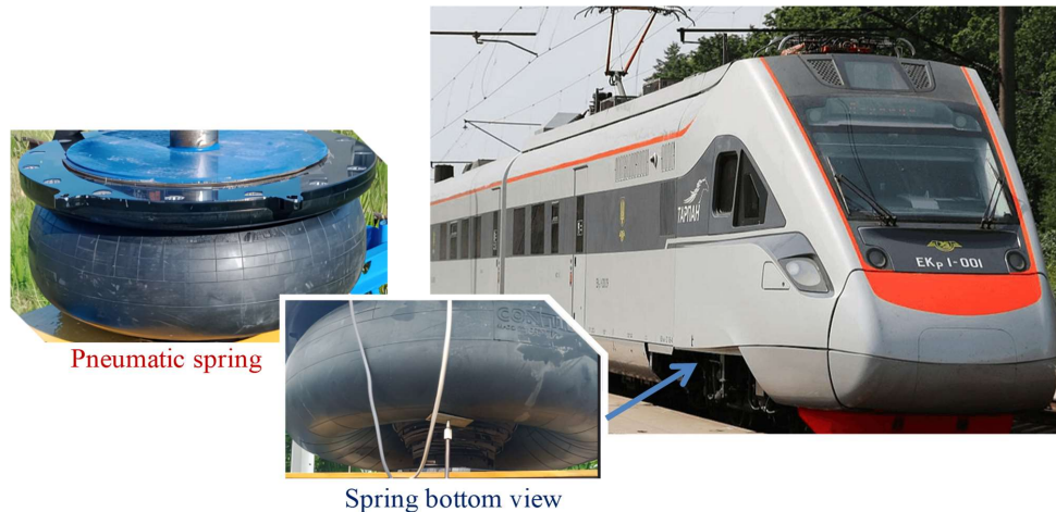
Fig. 1. Pneumatic spring for high-speed rolling stock
