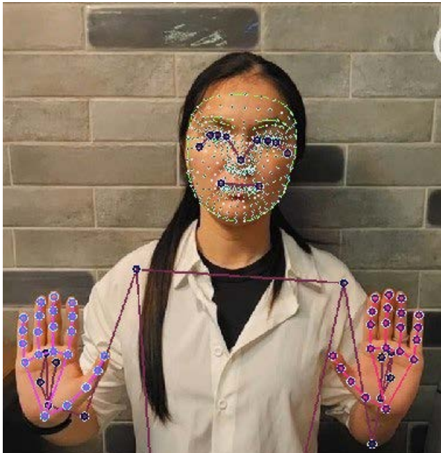
Fig. 2. Displaying face and hand landmarks using Mediapipe Holistic and Mediapipe Drawing Tools
