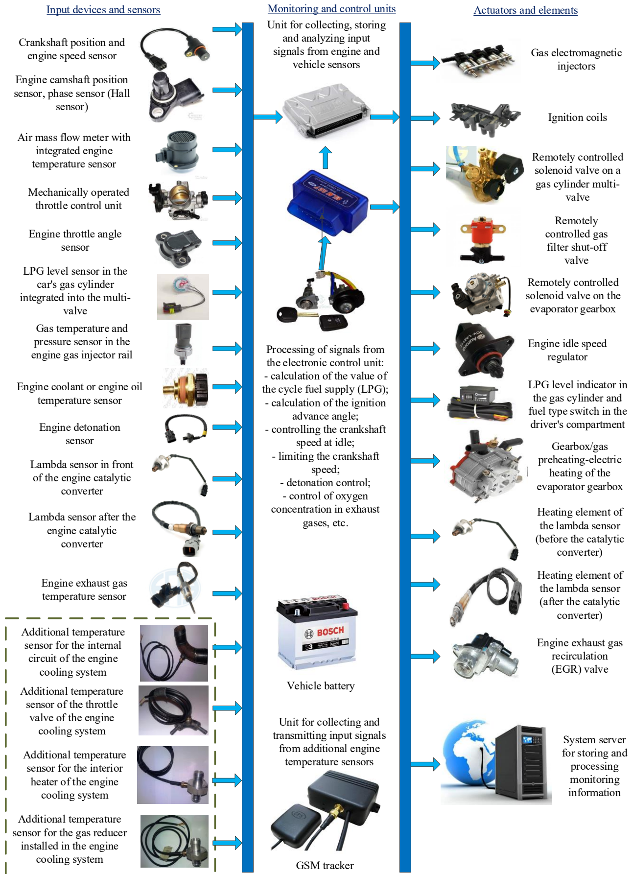
Fig. 1. Functional diagram of the interaction between the standard vehicle engine control system and elements of the remote monitoring system for thermal readiness processes
