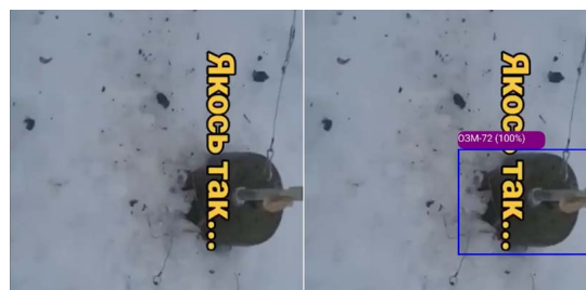
Fig. 3. Two frames from a video displaying an OZM-72 landmine, processed through the application, are nearly indistinguishable.
