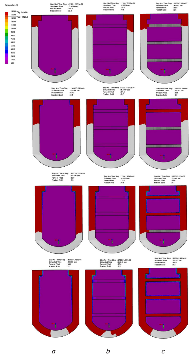
Fig. 5. Temperature fields (cross-section of the cell) during pouring: a – casting with functional material, b – casting with reinforced filler, c – casting with functional filler, which is reinforced from the liquid phase of the shell metal
