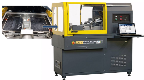
Fig. 5. Installation for testing the rutting resistance of asphalt concrete slab samples
