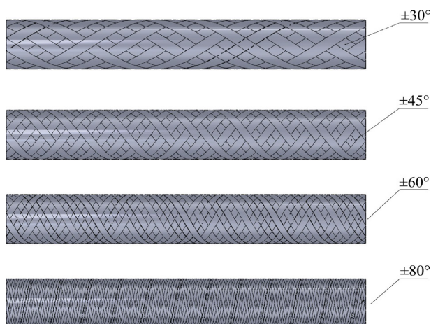
Fig. 2. Samples of carbon fiber reinforced plastic tubes with different winding angles
