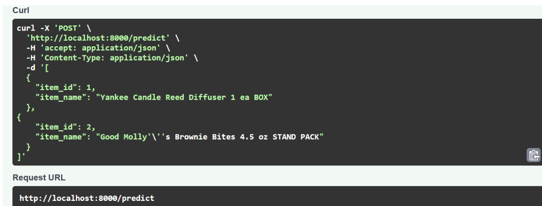
Fig. 3. Example of an HTTP POST request to API for categorizing products by hierarchical structure, executed in the Postman system using a local categorization model server
