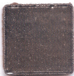
Fig. 10. The external condition of the surface of sample No. 19, formed using the electron beam surfacing technological mode: beam energy density 40 \text{ J/mm}^3 and its movement speed 500 \text{ mm/s}
