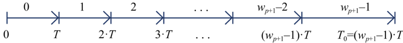
Fig. 2. Bounds of numerical intervals for different modules of the residual class system
