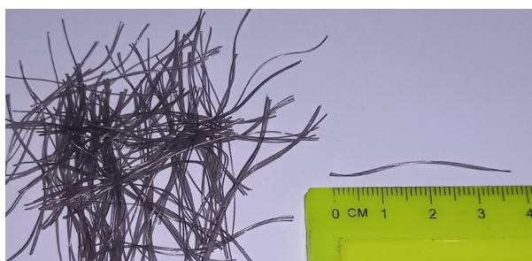
Fig. 1. X Mesh polypropylene fiber with a fiber length of 39 mm and an equivalent diameter of 0.45 mm
