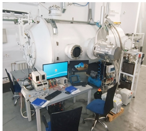
Fig. 3. General view of the vacuum chamber in which experimental studies were conducted
