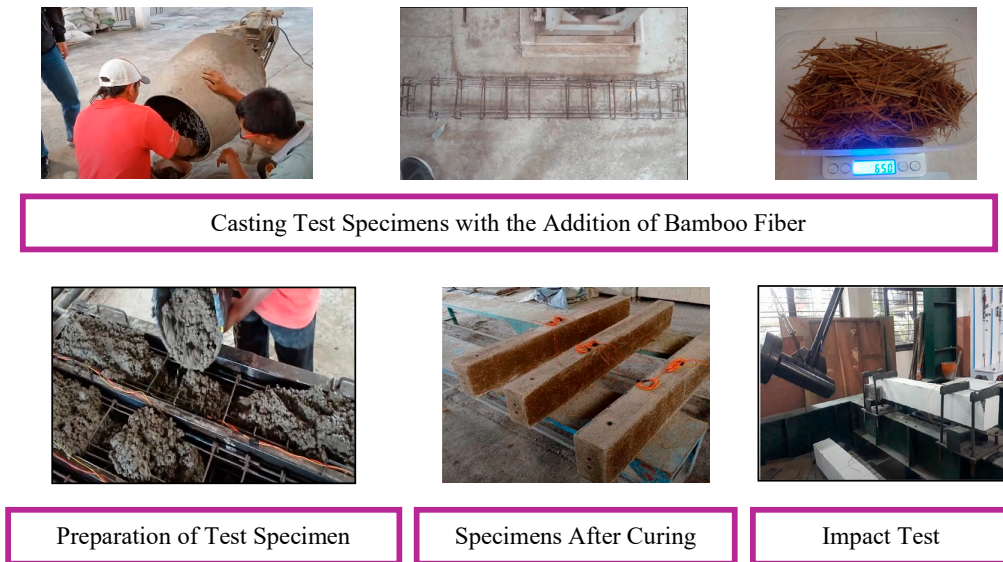
Fig. 4. Schematic of casting test specimens with bamboo fiber addition and impact testing
