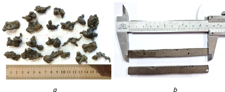
Fig. 1. The local content sample: a – ferronickel shot; b – ferronickel blocks
