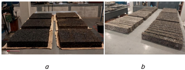
Fig. 2. Preparation TPB test: a – slab specimens; b – beam specimens
