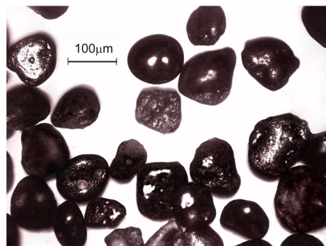
Fig. 1. Grains of Samotkan ilmenite concentrate. Carl Zeiss Jena NU-Microscope
