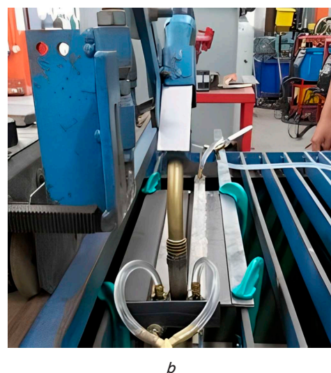
Fig. 1. Schematic illustration of: a – heat sink and clamp; b – experimental setup of welding
