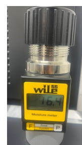
Fig. 4. Measurement of nut moisture using Wile 55 moisture meter
