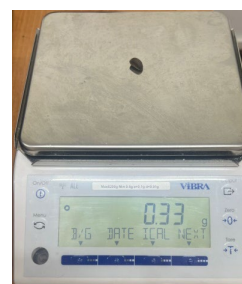
Fig. 3. Measurement of nut mass using Vibra ALE-6202R scales
