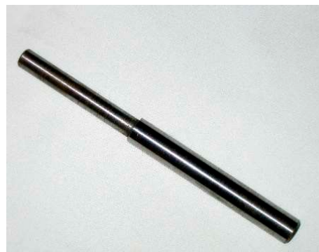
Fig. 11. Movable steel finger for wear testing
