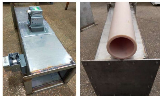
Fig. 3. Resonator shaft: a – with built-in magnetrons; b – with a radio-transparent reactor
