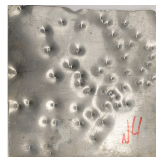
Fig. 3. A sample of damage to a duralumin plate 1 mm thick with a shot diameter of 3.75 mm, shot weight of 42 g, and powder charge weight of 1.65 g
