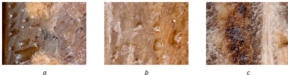
Fig. 10. Results of LB observation with a 3D microscope at 200x magnification: a – NaOH 2%; b – NaOH 4%; c – NaOH 6%
