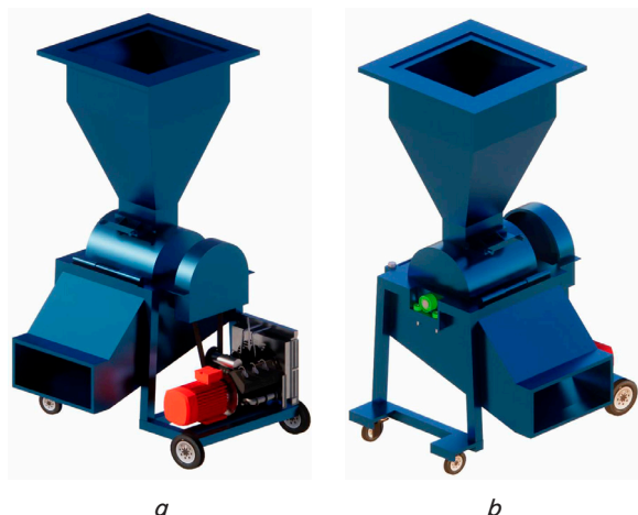
Fig. 3. Portable machine for recycling the CDW into fine aggregate: a – right side; b – left side
