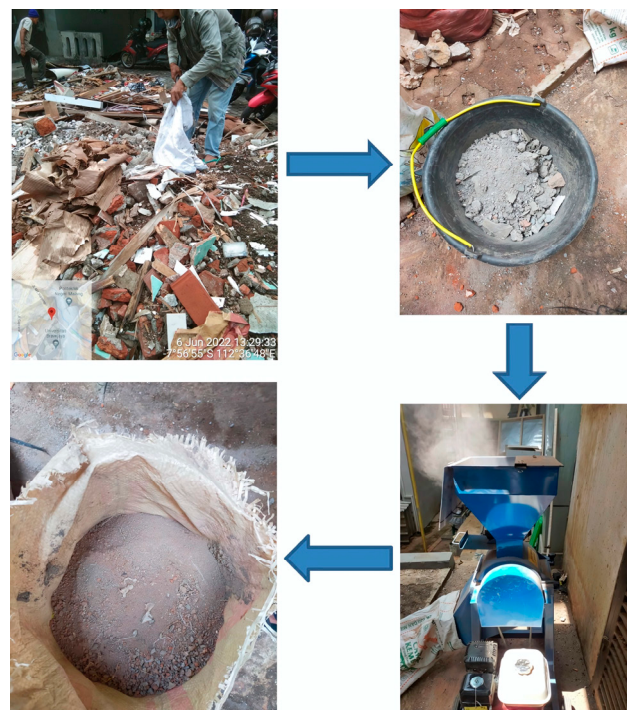
Fig. 8. Sand substitutes aggregate process from CDW: a – raw debris; b – debris after crushing by hammer; c – aggregate crusher machine; d – sand material for reuse
