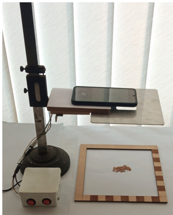
Fig. 1. Laboratory bench for photographing grain samples
