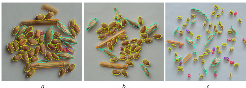
Fig. 2. Annotating images using the Roboflow Annotate interface: a – with dense placement of objects; b – with partial overlap of objects; c – with a variable distance from the camera lens to the material sample
