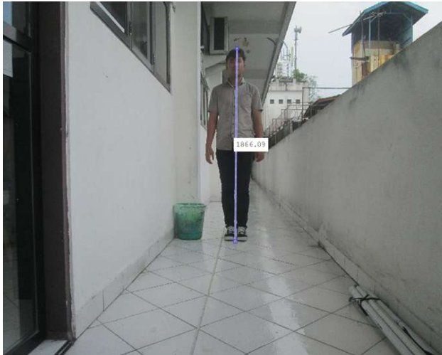
Fig. 3. Measurement of the distance to person object at 3.4 meters: 1866 pixels
