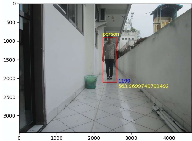
Fig. 6. Results of YOLOv3 distance measurement predictions
