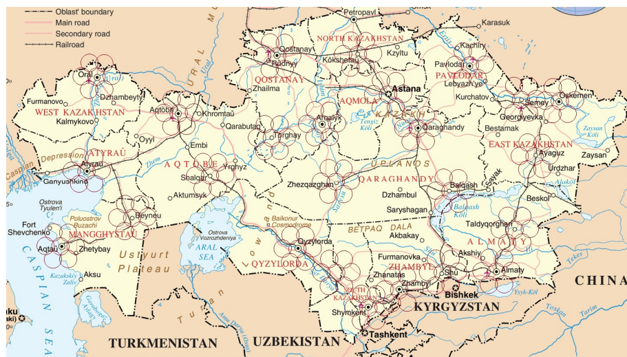
Fig. 3. The scheme of the calculated placement of a network of stratospheric airships on the territory of the Republic of Kazakhstan to ensure wireless communication
