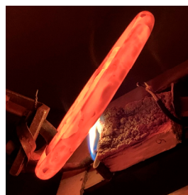
Fig. 1. Model sample of wood treated with a biocomposite coating with the addition of potassium nitrite
