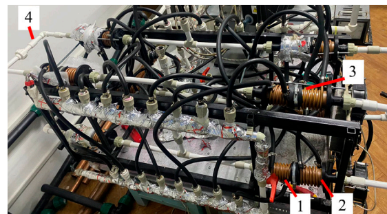
Fig. 1. Photograph of a laboratory prototype of a thermoacoustic Stirling engine: 1 – cold heat exchanger; 2 – hot heat exchanger; 3 – stage with heat exchangers and regenerator; 4 – tubular resonator
