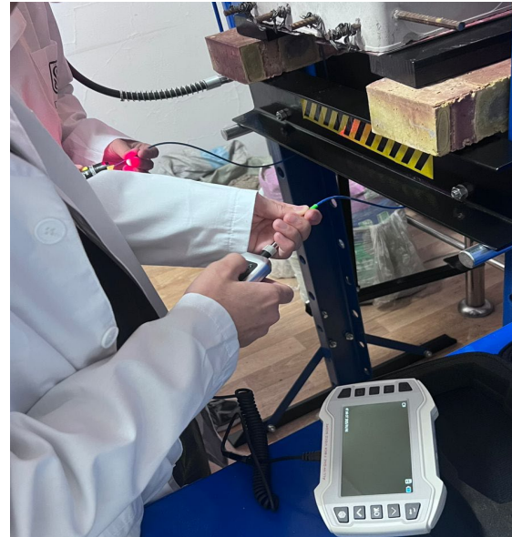
Fig. 2. General view of the experimental setup with optical interrogator, fiber-optic channel connection, and hydraulic press
