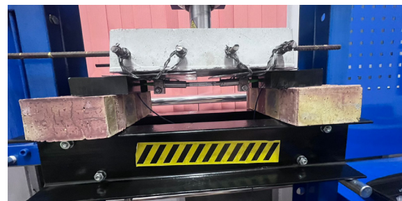
Fig. 3. Crack propagation on the specimen surface after maximum load
